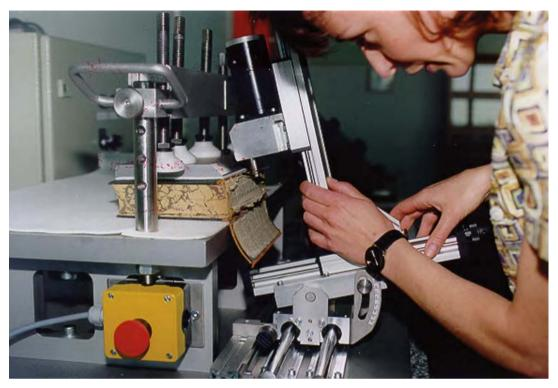
Figure 21.9 The board slotting machine developed by Becker Preservotec in cooperation with the Academy of Art and Design, Stuttgart.
