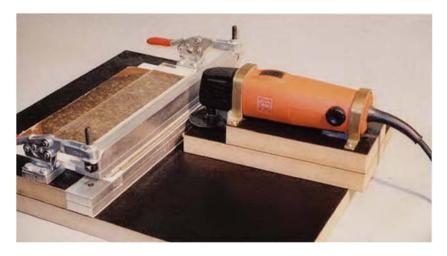
Figure 21.11 Minter's mounted FEIN MultiMaster with oscillating saw blade for board slotting is advanced by hand to create a slot in the edge of the binderboard which is clamped in the jig.
