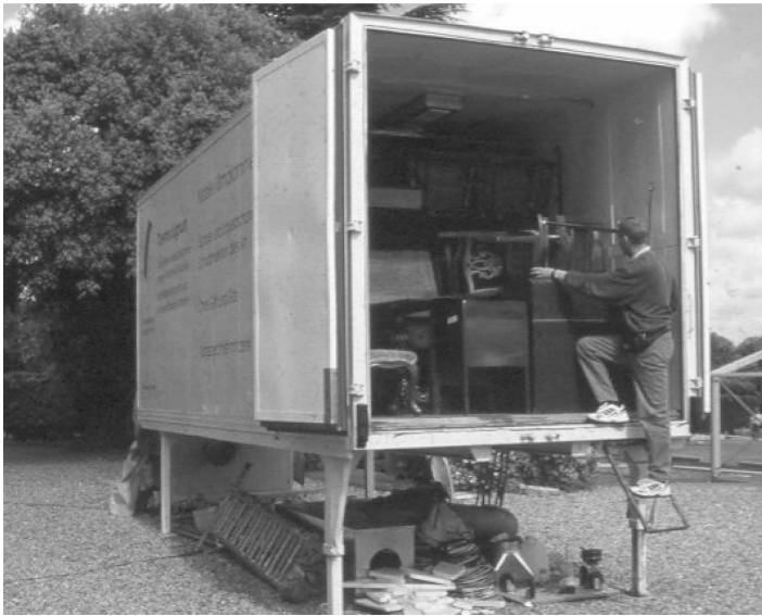
Figure 2. Mobile Thermo Lignum unit heat treating furniture at a historic house.
