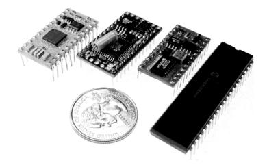
Microcontrollers are small and cheap. This allows you to explore location-specific projects that embed computers in the most unlikely places, like shrubbery and sneakers, or to develop projects where the actions of many simple devices add up to a more interesting whole.
