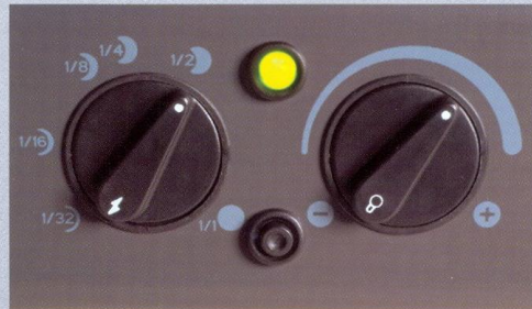
Independent modelling lamp and flash power controls (5-stops range) on a Bowens Esprit monobloc; charge indicator lamp and flash dump button in between.
