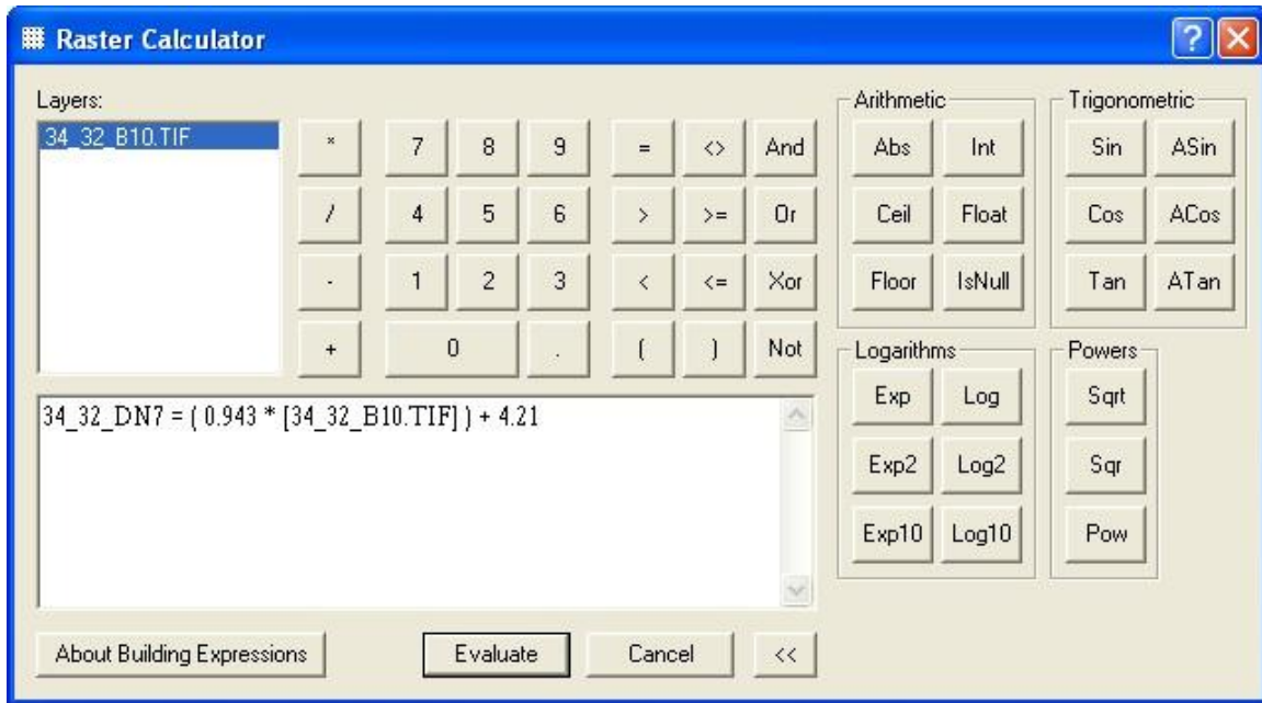
Figure 3. Raster calculator function to perform the transformation from Landsat 5 TM DN data to the equivalent Landsat 7 ETM+ DN data
