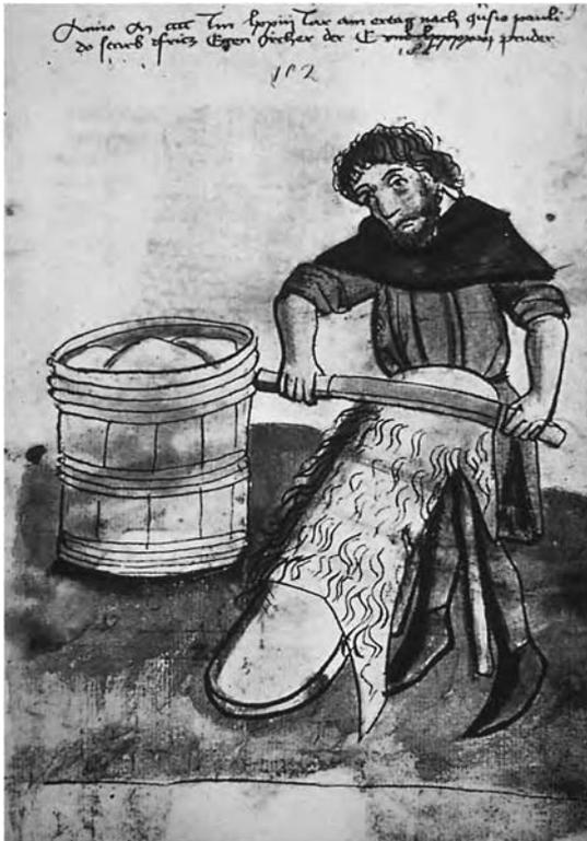
Figure 7.4 Removing hair with two-handed knife.
