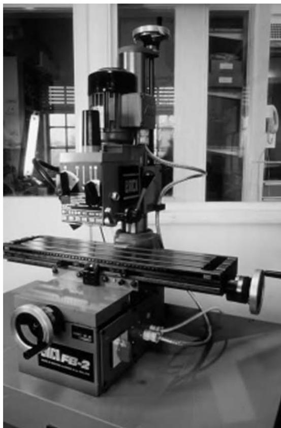
**Figure 21.8** The milling machine Emco FB-2, used for the board slotting technique by the Bodleian Library.
