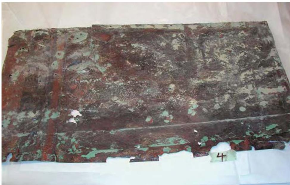
**Figure 23.94** Back of panel 4 showing contact adhesive, paint and plaster.
