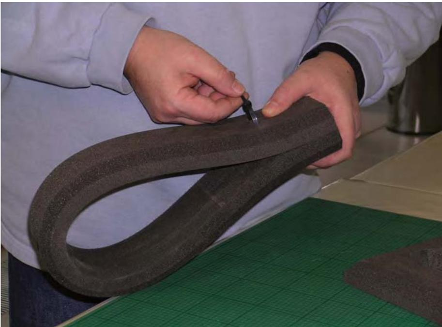
**Figure 23.50** The cable tie is threaded through the holes tightened and the excess tie cut off.
