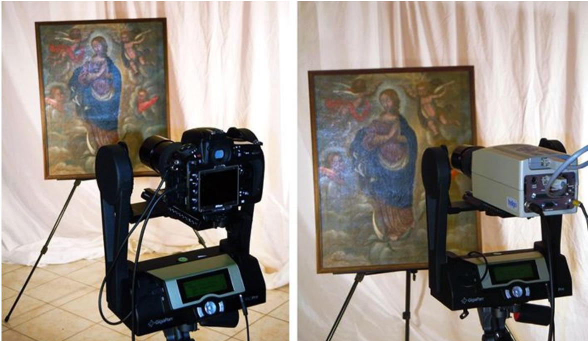
Figure 8. Gigapan EPIC Pro Panoramic head with Nikon D800 (left) for multispectral imaging and with InGaAs camera Merlin Indigo Systems (right) for Infrared Reflectography, both mounted with a Nikon Nikkor 200mm lens.
