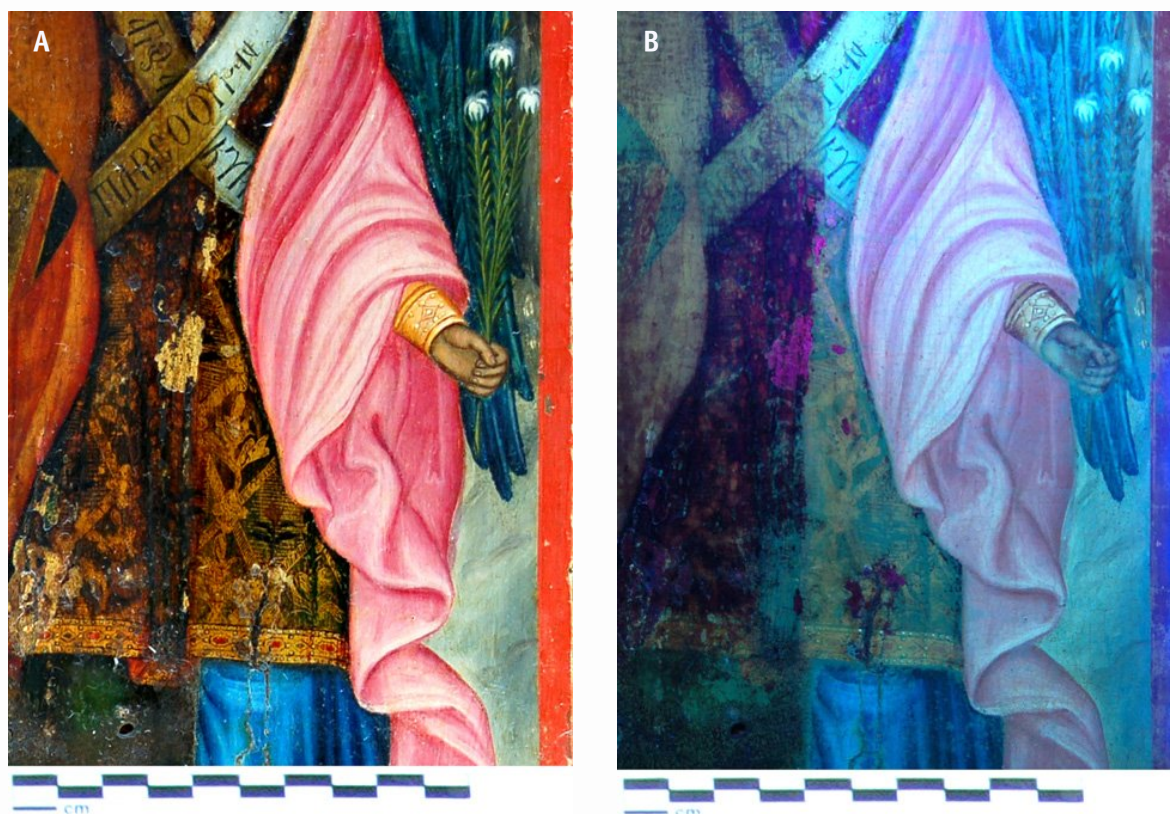
Figure 9. Visible (a) and UV fluorescence (b) images of the gilded part of the clothing of Archangel Gabriel as unsoiling with the HPMC hydrogel (gel A) was in progress. The left part of the gilded surface demonstrates the obscuring problems introduced by the soiled and discolored varnish, while at the right part the improvement of the area appearance is obvious. The successful soiling removal is confirmed by UV fluorescence (b). Note that varnish of the surrounding painted surface was removed earlier with organic solvents.
