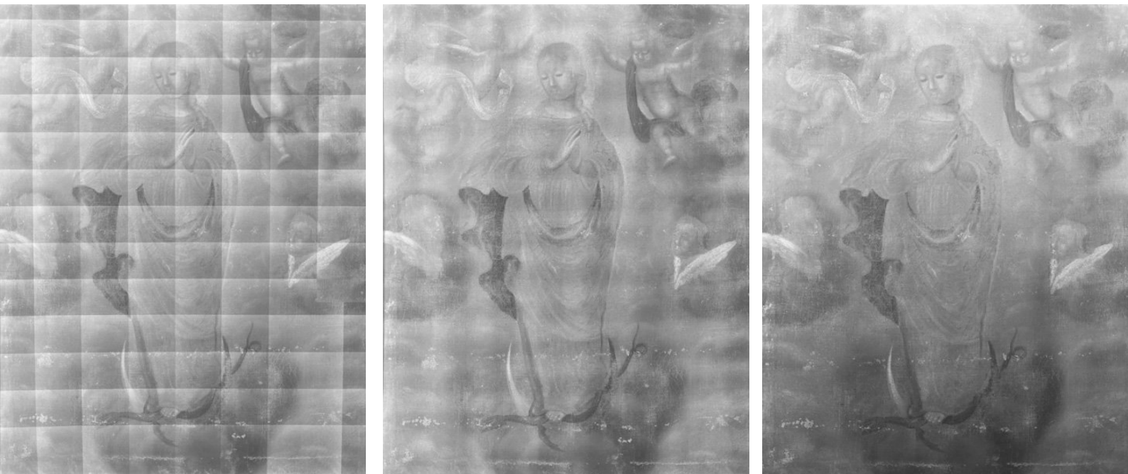
Figure 6. a) 104 images tiled (overlapped) without any blending; b) PTGui panorama without vignetting correction; c) PTGui panorama with PTGui vignetting correction.
