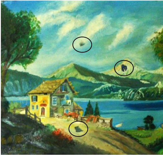
Figure 2. The oil painting model after applying three soot specks on its surface, namely in the central cloud, in the right mountain and in the road.
