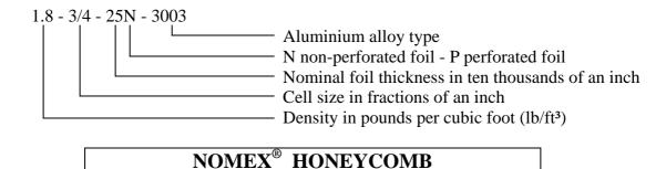
Technical Resin Bonders can supply cut slices of aerospace and commercial grade Nomex<sup>®</sup> honeycomb in a range of densities to suit individual customer requirements.
