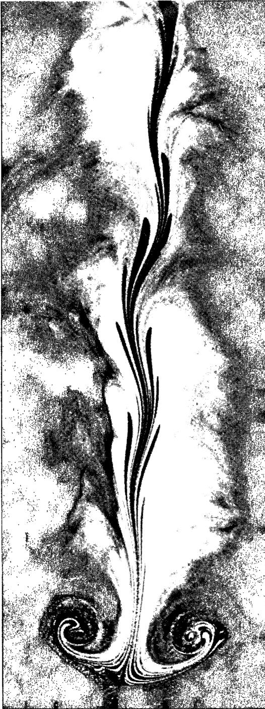
CHAOTIC FLOWS. A rod drawn through viscous fluid causes a simple, wavy form. If drawn several times, more complicated forms arise.
