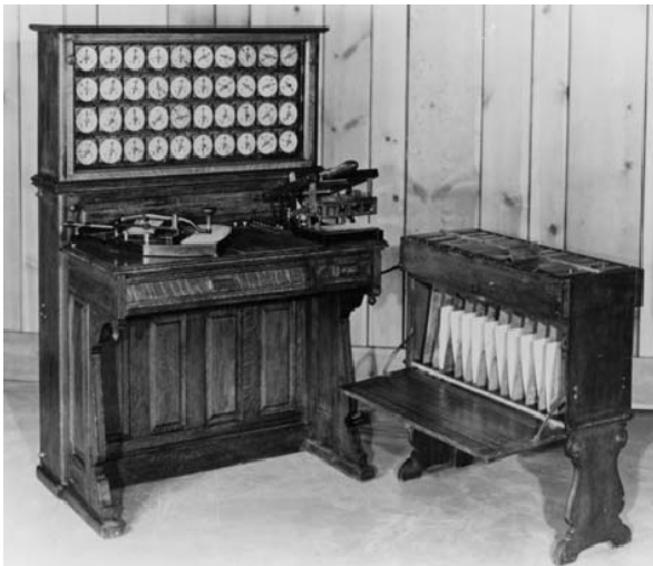
Fig. 2.33 Hollerith’s punched card tabulator. With kind permission of IBM, Corporate Archives, Somers, NY.
