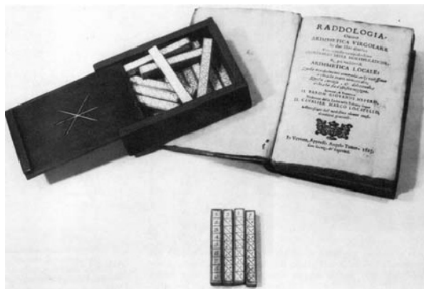
Fig. 2.14 Napier’s rods and title page of a calculating instruction by Lord Napier, translated into Italian, Verona 1623 [4, p. 17].
