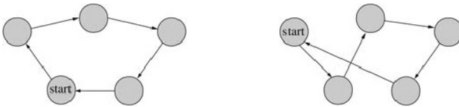
Fig. 10.5 Two solutions of a Nearest Neighbor Heuristic for the Traveling Salesman Problem
