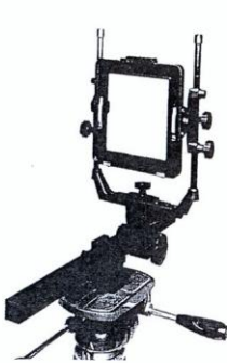
The front standard can move along the rail, and contains the mechanisms for adjusting the position of the lens it is designed to support.
