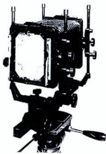
The camera back clips into the rear standard and contains the spring back to hold the film and the ground glass to allow focusing.
