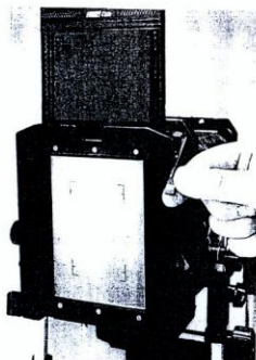
A bail lever is sometimes incorporated into the spring back to facilitate the insertion of film holders.
